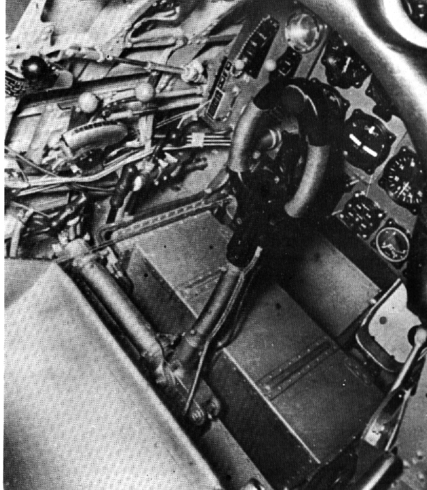
Left side view of the He 112 cockpit.
