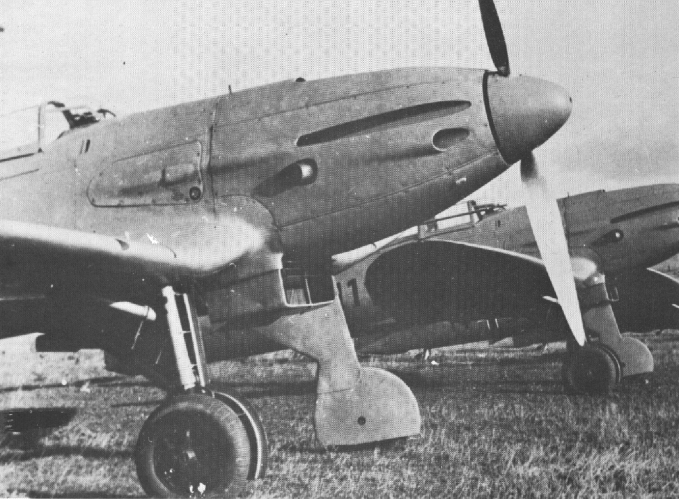
Location of armament in wings and engine cowl and maintenance access panels are illustrated in this photo of He 112 B-O's in Luftwaffe markings.
