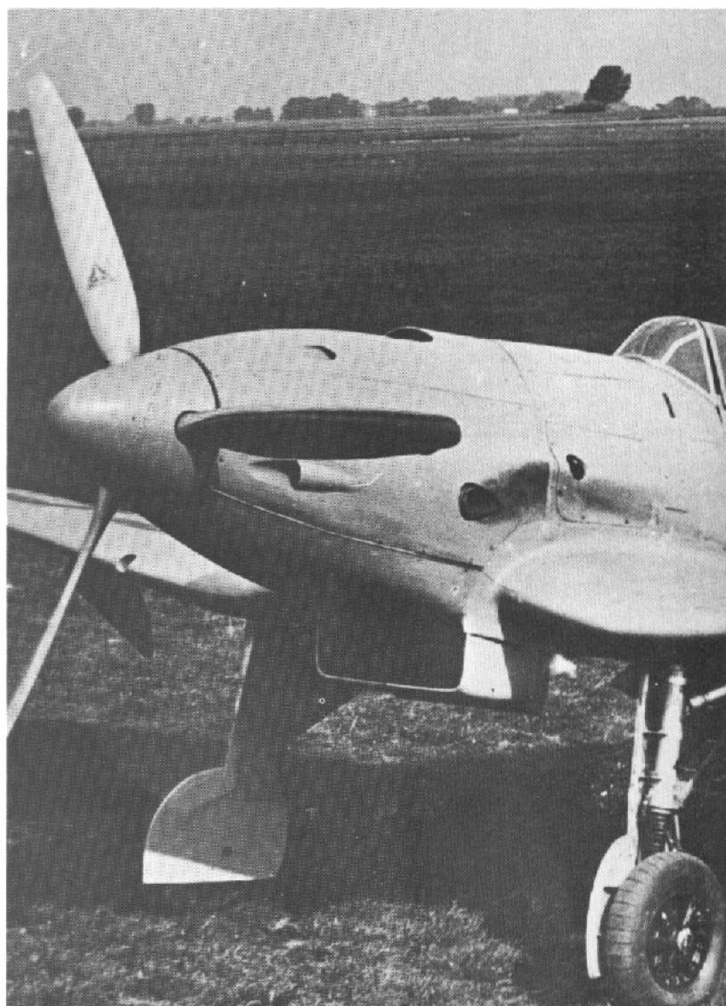
Close up of the V-9 shows the retractable radiator and the wide track undercarriage.
